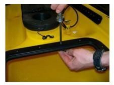
6. Installing the lid. Place the lip under the front of the hatch ring as shown below.
