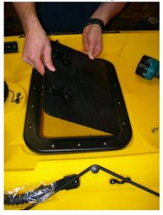
Then push down and turn the knobs and lock down.
