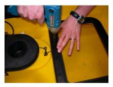
4. Place the hatch ring over the cutout, (should be a snug fit), and drill out the screw holes with the 13/64<sup>th</sup> drill bit. TIP- drill 2 holes on opposite sides and install a nut & screws in each then drill out the remaining holes.
